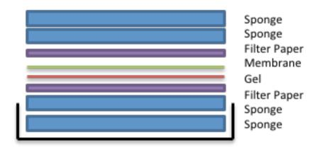
Cathode Chamber of Blot module
