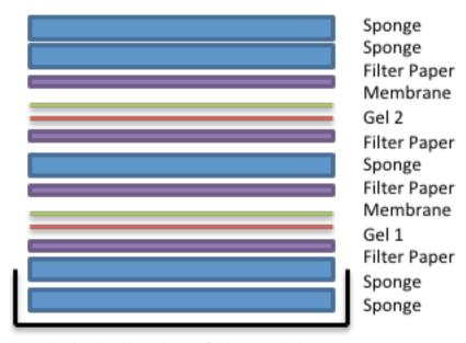
Cathode Chamber of Blot module
